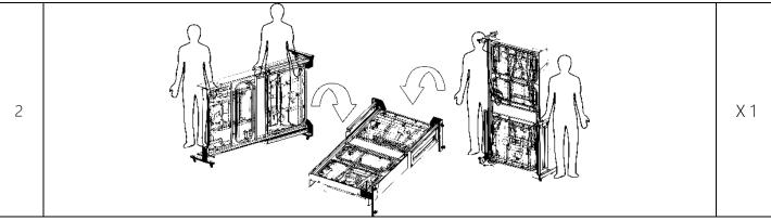
Using two persons, lower bed from either the horizontal or vertical transport positions to the normal use position
